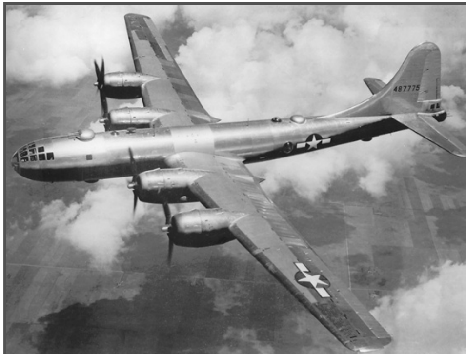
A B-29 Superfortress soars through the air over Marietta, Ga. The Superfortress was a four-engine propeller-driven heavy bomber designed by Boeing that was flown primarily by the United States toward the end of World War II and during the Korean War. Marietta Army Airfield performed acceptance testing for the B-29s. (Courtesy photo)
