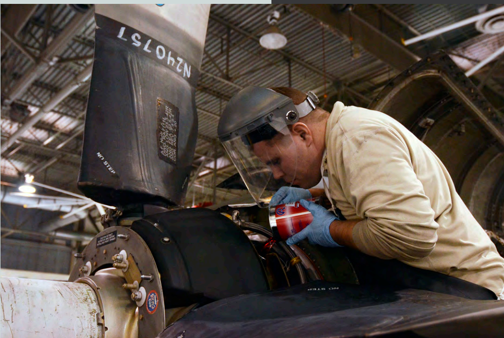
(Far left) Tech. Sgt. Rafael Zeruto, 94th Aircraft Maintenance Squadron propulsion supervisor, and Tech. Sgt. Trent Morris, 94th AMXS propulsion technician, reinstalls a propeller on a recently acquired C-130 H3 aircraft. Maintenance personnel are transitioning seven C-130 aircraft from H2 to H3 models, tasked by Air Force Reserve Command to be completed by July 2014. (U.S. Air Force photo/Don Peek)
