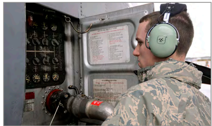
Airman 1st Class David C. Yancey, 94th Maintenance Squadron crew chief, monitors the indicator panel of a C-130 Hercules aircraft during a fuel transfer March 3. Dobbins recently switched from JP-8 to Jet A fuel, along with other units, projecting to save the Air Force millions of dollars annually. (U.S. Air Force photo/Don Peek)
